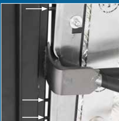
Steel pins provide the same resistance as real locks
