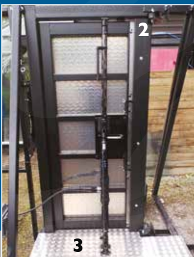
Steel pins provide the same resistance as real locks
